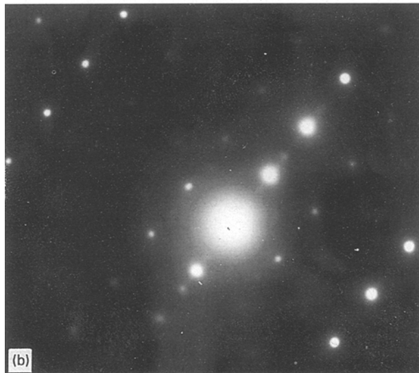
Figure 9 (a) Bright-field transmission electron micrograph showing the needle-shaped Al-Cu precipitates, in the T6 condition, of the unreinforced matrix material. (b) Corresponding selected-area diffraction pattern taken from the same region.
